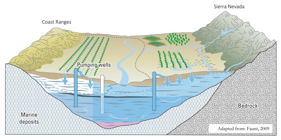
Figure 3-3 Generalized Cross-section of the San Joaquin Valley
