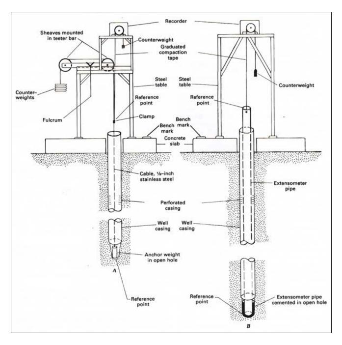
Figure 7 – Simplified Extensometer Diagram
